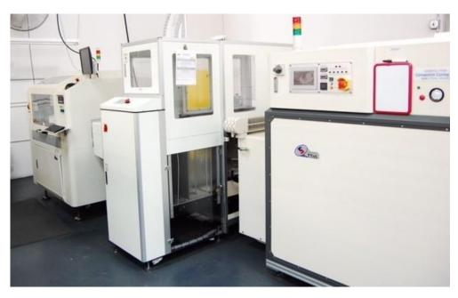
SoPark's robotic selective coating system with large 15.75 in. X 22.0 in. capability.
